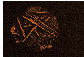
Electron microscope image of ammonium sulfate crystallized on the leaf surface after an application with a typical APG based nonionic surfactant/ammonium sulfate blend.
